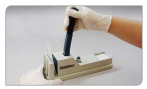
**Step 2:** Lift the handle and insert the pouch between the crushing plates.
